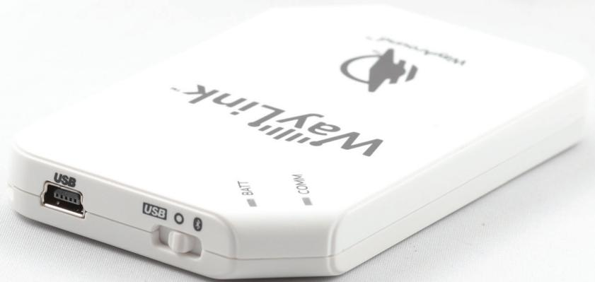
On the right side is a push button to wake up the WayLink if it has gone to sleep. When active, the WayLink will remain charged for 5.25 hours or 6,345 NFC scans.
